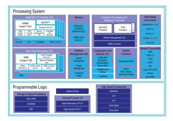
Applications processing unit (APU) with quad-core ARM® Cortex<sup>™</sup>-A53 processors up to 1.5GHz:
